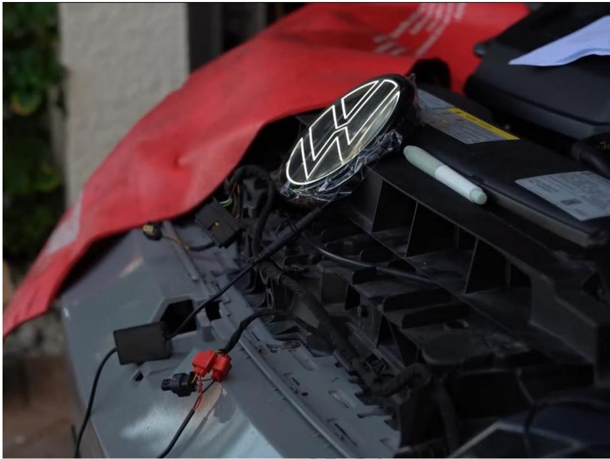
5 Remove factory emblem from rear of grille. Use a plastic trim tool or flat screwdriver to push the clips outward.
