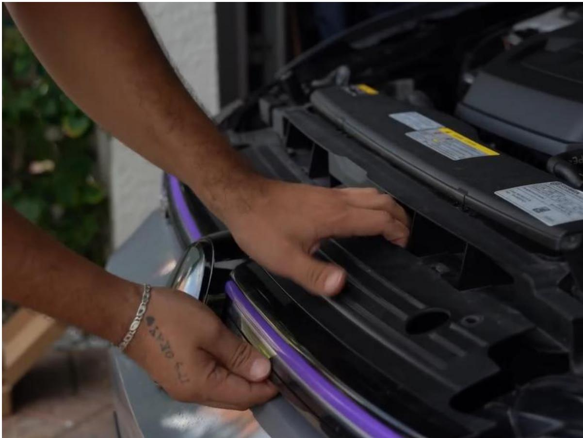
2, Behind the grille, locate and unplug 3 connectors. Left light bar connector, Right light bar connector and ACC radar-related connector. Press the locking tab and then Pull the connector straight out.
